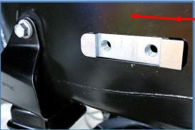
11. Place the reservoir bracket over the backing plate and install the two 8mm bolts (CB3825) into the backing plate and tighten bolts using a 12mm wrench or socket. See final install pics for proper orientation.
