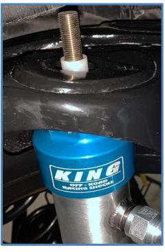
5. Place the upper bushing on the mounting stud followed by the blue retaining washer, 1/2" washer and nut. Apply anti-seize to the threads and thread the nut on finger tight for now to hold the shock in place.
