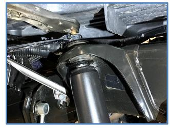
3. <u>Install Brake Line Bracket</u> – Remove the bolt holding the factory brake line bracket using a 12mm socket. Attach the provided Brake Line Bracket to the factory location using the factory bolt, then attach the factory brake line bracket to the new bracket as shown below using the supplied 8mm bolt (CB3825) place the supplied washer and nut on the bolt and tighten.
