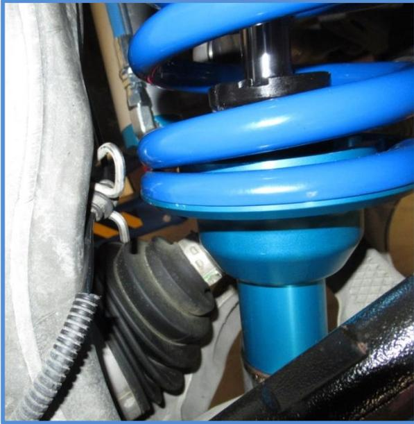
18. Place the tires on the vehicle and tighten lug nuts. Remove jack stands and lower vehicle to the ground. With the vehicle sitting on the ground, torque the lower mounting bolt to factory specs.
