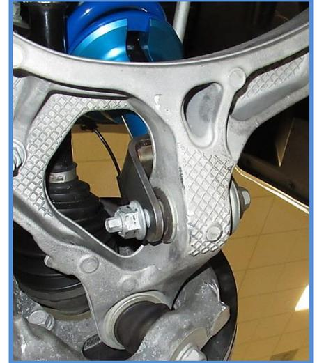
12. Reconnect the upper control arm and torque nut to factory specs.
