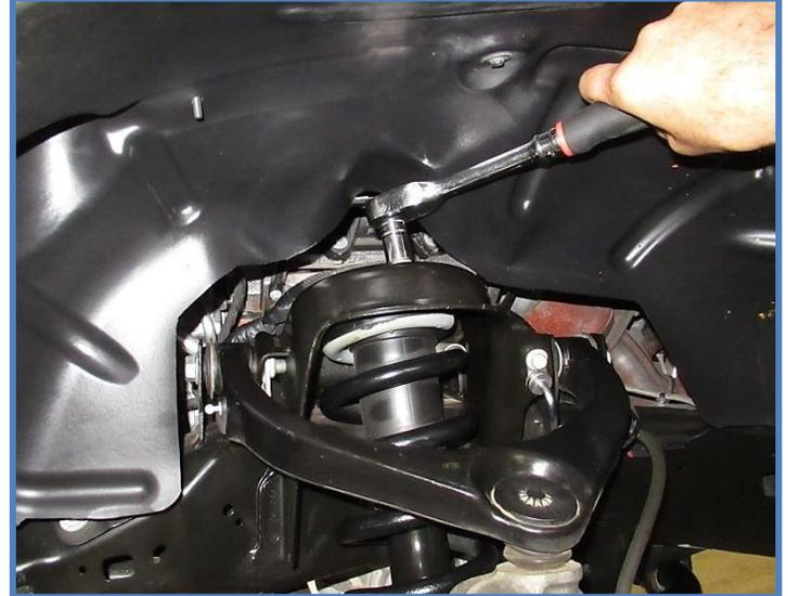
3. Disconnect the upper control arm. Remove the nut using a 21mm socket and separate a-arm from knuckle.
