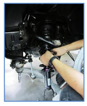
3. Install King Shocks by placing them in position on the vehicle and install the factory bolt in the lower mount but do not tighten yet. Be aware that the shocks are side specific and should be positioned so that the hose is pointing towards the front of the vehicle.
