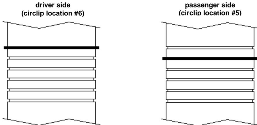
Another example: to achieve the highest lift setting of 1.75" on a **4x2 V6 Double Cab 5' bed**, the circlips should be installed as follows:
